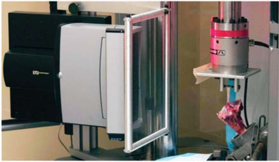
Figure 2. Biomechanical test setup with the advanced video extensometer (left) and customized alignment fixture (bottom right), which allowed for the force vector to be applied in line with the tibial tunnel.
