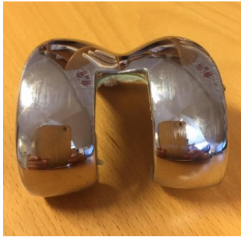
Fig.10 Private photo of extracted femoral component after revision surgery, demonstrating a deep trochlear groove with elevated lateral flange, so-called patellar-friendly design.
