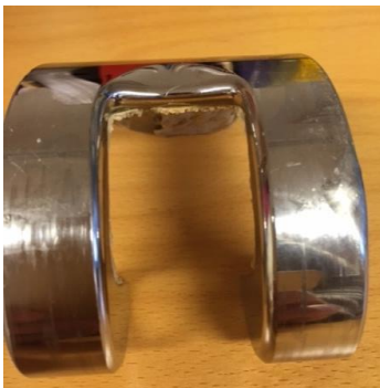
Fig.9 Private photo after revision of knee arthroplasty implanted in 1989 in Haugesund Rheumatism Hospital in a rheumatoid patient. The femoral component has a non-existing trochlear groove and therefore so-called patella-unfriendly design. The implant was known as Accord, the Johnson/Elloy concept by Thackray.
